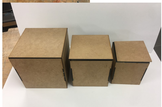
Creating models using CAD and cutting them on the laser cutter helps produce models/maquettes of the highest quality. The design below helped decide on the size of outcome.
