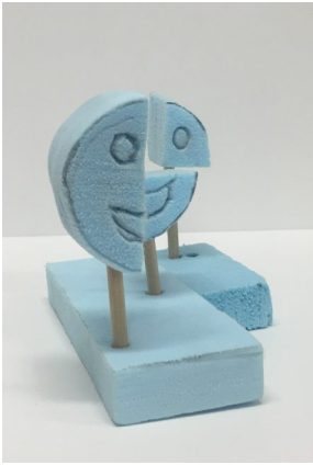
Testing design ideas in foam is quicker and helps you develop the idea.
