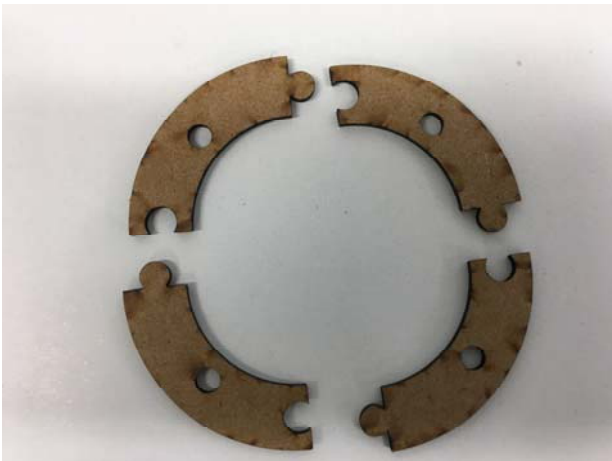
Testing parts on the laser cutter in MDF first.
