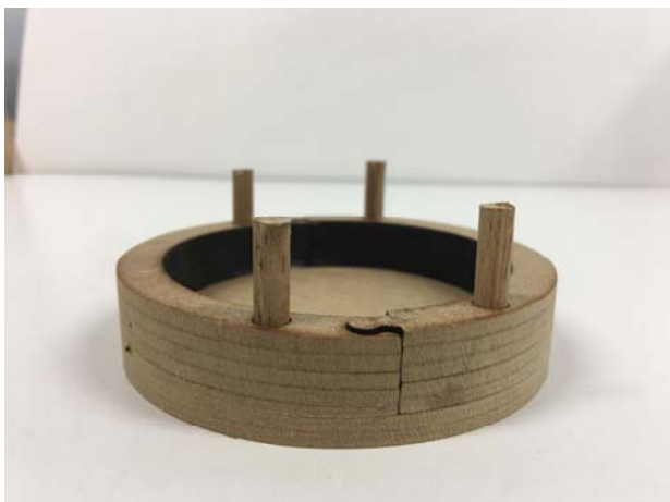
Testing parts on the laser cutter in MDF first.
