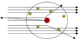
Rutherford experiment: Most alpha particles travel straight through the gold leaf, some are deflected (change direction) and very few are completely bounced back towards the source. This provides evidence of a central area of high positive charge in the
